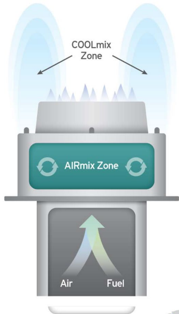
Figure 3-2. Schematic of John Zink Hamworthy SOLEX Burner
