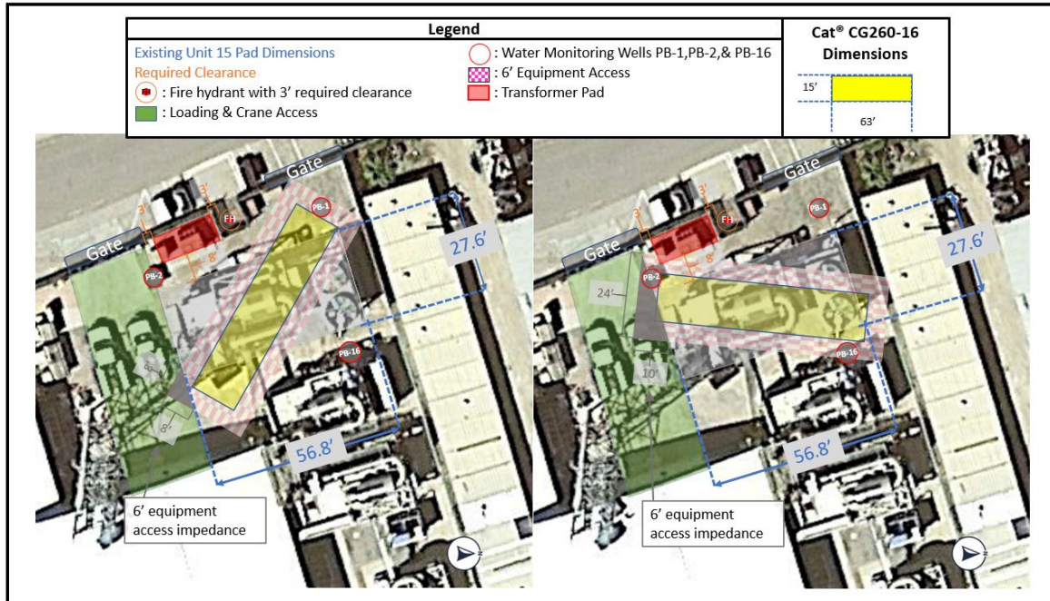
Figure 1. Caterpillar Model CG260-16 Rotated Approximately 45 Degrees Counter-Clockwise (Left) and Approximately 40 Degrees Clockwise (Right) with Respect to Existing Unit 15's Orientation.
