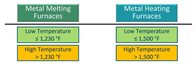
**Note:** Rule 1147 uses 1,200 °F to establish low and high temperature cutoffs for both metal melting and metal heating furnaces
