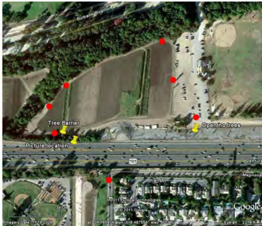
Figure 2. Proposed stopping locations for collection of average data (shown in red) based on the anticipated southeast winds. Also shown is the proposed upwind sampling location.
