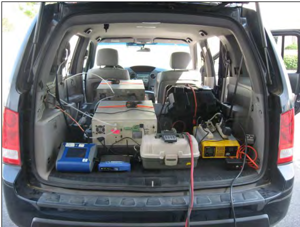
Figure 2-3 Instrumented Sampling Vehicle Operated by T&B Systems
